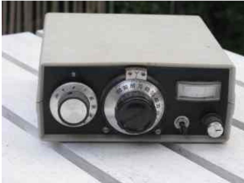
The photo above shows the completed L-match and resistive bridge. The variable capacitor adjustment is in the centre of the front panel. To its left is the ten-position rotary switch for the adjustment of the L-match inductor. The right-hand third of the panel is taken up by the resistive antenna bridge. Below the meter movement is the tune/operate switch and the meter's sensitivity control.
