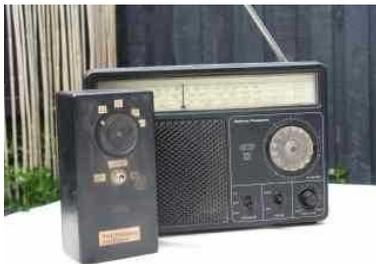
Since most amateurs switched from AM to single sideband more than 40 years ago, it hasn't been possible to receive them with an unaided shortwave receiver. All you'd hear is garbled 'duck talk'. Here's the solution. It's a one-transistor beat frequency oscillator that makes 3.5 and 7 MHz amateur SSB signals intelligible on a cheap receiver.
